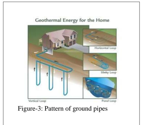
Figure-3: Pattern of ground pipes
