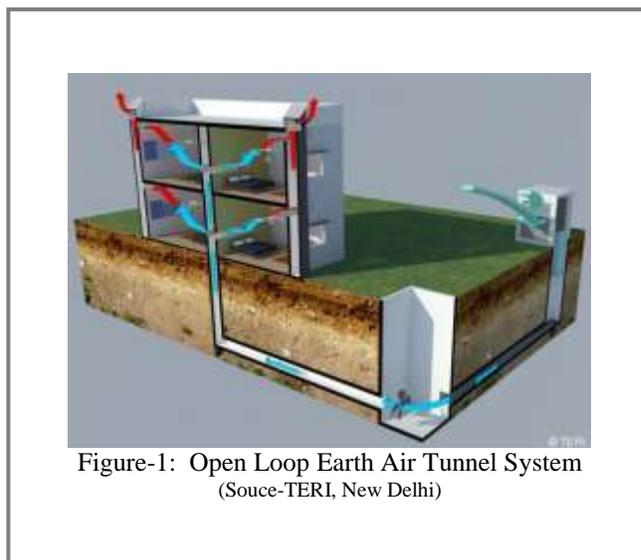
In open loop system, Outdoor air is drawn into EAT and delivered to the inside of the building. Hot air from inside of the building is exhausted through solar chimney. Illustration of an open loop cycle is at Figure-1:
