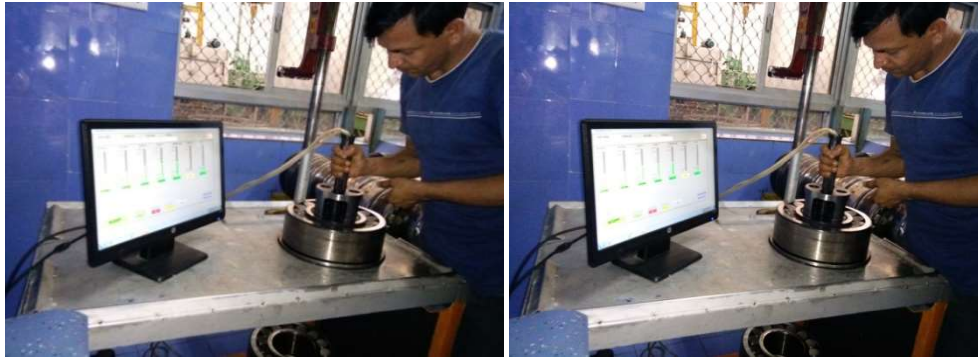
Measuring Bore Diameter of Roller Bearing.
